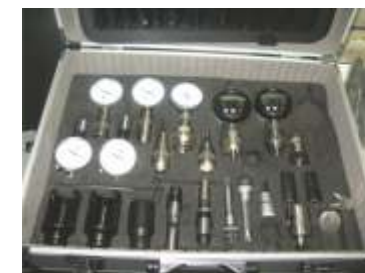
Cmx 108 SET OF SPECIAL TOOLS FOR DISASSEMBLING, ASSEMBLING AND MEASUREMENT OF BOSCH COMMON RAIL INJECTORS
