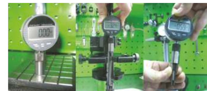
170-0945/2 BOSCH NOZZLE NEEDLE STROKE MEASURING TOOL
