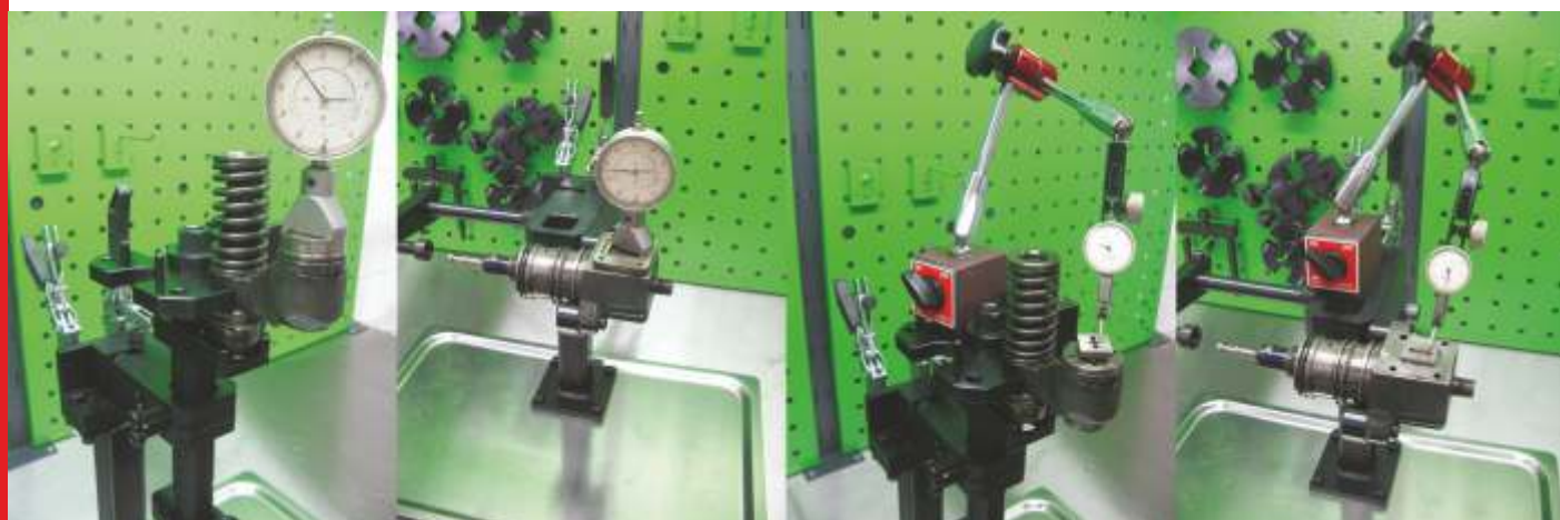
MAGNETIC GAP MEASUREMENT
