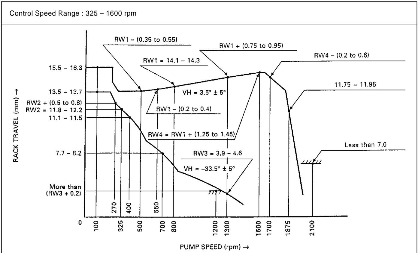
6. ADJUSTMENT OF BOOST COMPENSATOR (Full lever position)
