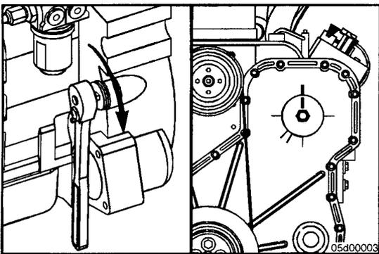
After removing the front access cap, rotate the engine using the turn over tool until the Timing mark on the pump drive gear aligns with the TDC mark on the timing cover.
