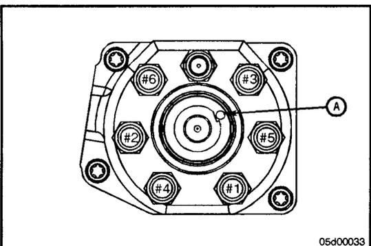
Check the position of the notch on the rotor. It should line-up with the alignment mark (A) on the outside of the distributor. If the alignment is correct the rotor is properly timed to the engine.
