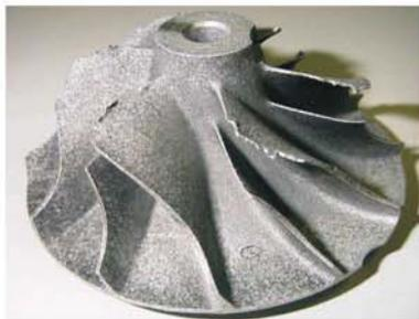
Salt or sand causes severe erosion and corrosion, eventually leading to blade failures.
