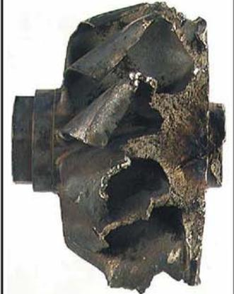
.....in extreme cases, the wheel can burst due to overspeeding. Minute stress cracks appear as the wheel is "stretched" beyond its designed limits and these gradually increase during overspeeding cycles followed by a final rapid failure.
