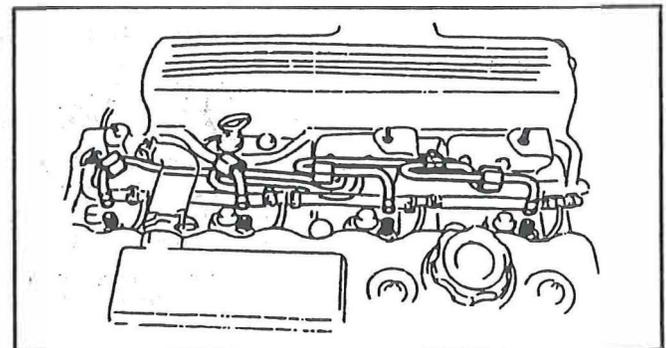
8. Crank the engine until fuel without air bubbles is discharged from the injector fuel lines.
