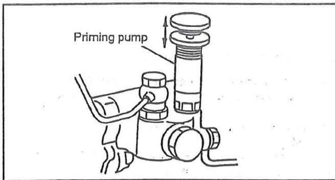
4. Next, loosen the injection pump's overflow valve, and pump the priming pump until fuel without air bubbles is discharged from the overflow valve. Close the overflow valve. Tightening torque: 1.2-1.5 kgm / (104-130 lbf in)
