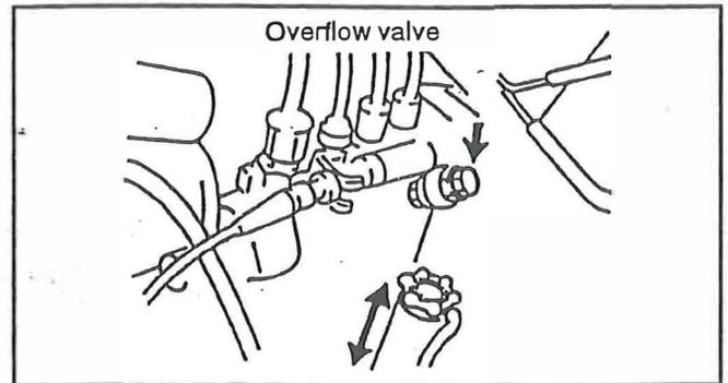
5. After bleeding the air out of the fuel filter and injection plug, press down the top of the priming pump plunger, and tighten it securely.
